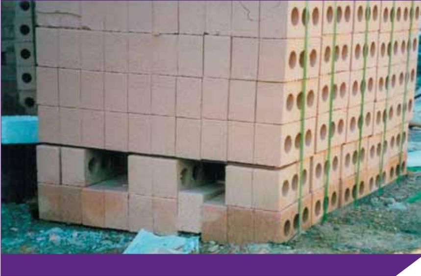
**Figure 1.** Staining from ground water
