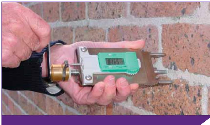
**Figure 18.** Scratch test performed on a mortar joint
