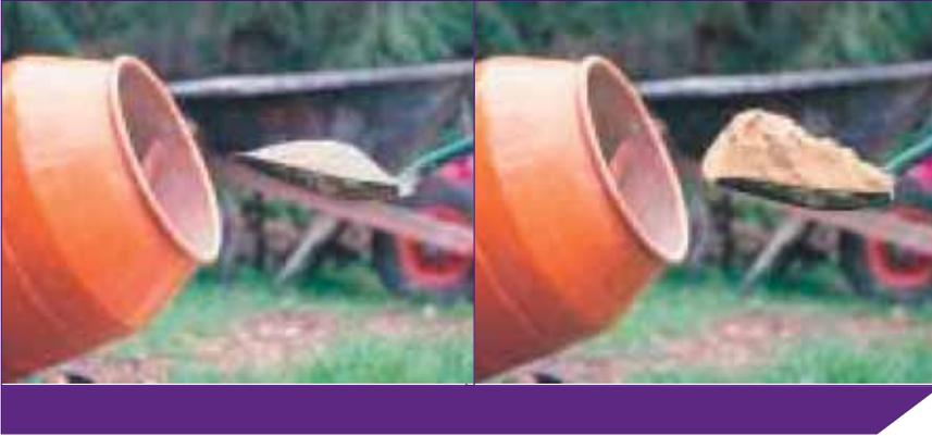
**Figure 5.** The effects of bulking on shovels of cement (left) and sand (right)
