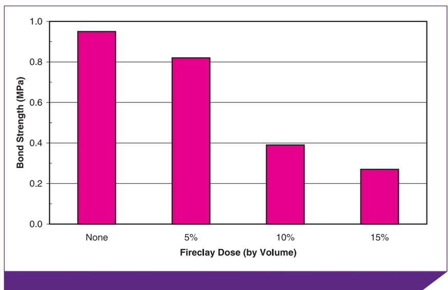
**Figure 3.** Typical effect on bond strength of using clay as a plasticiser
