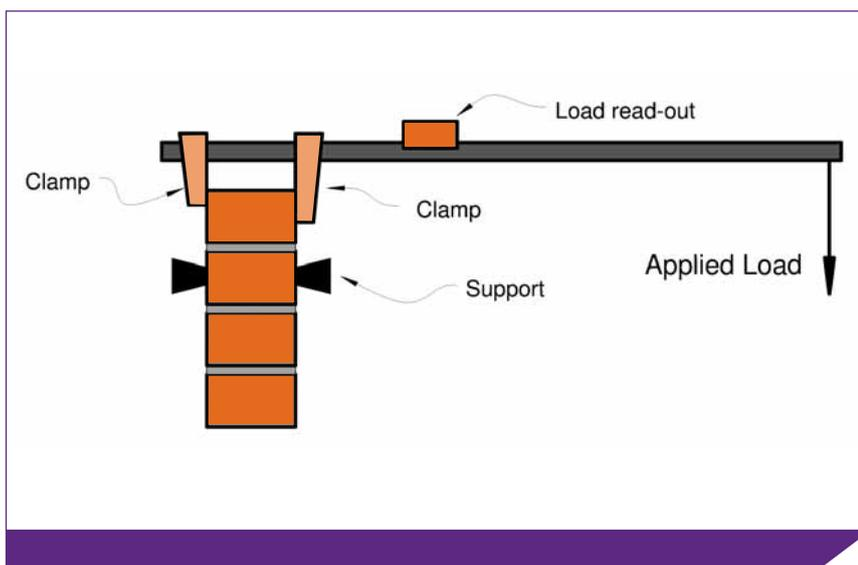
Figure 16. Schematic arrangement of bond wrench test
