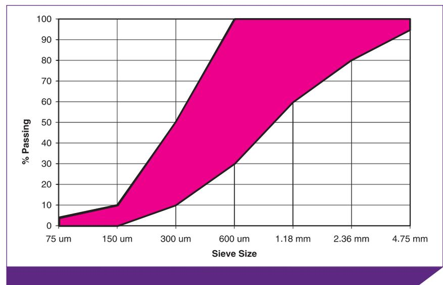
Figure 2. Typical sand grading envelope for mortar
