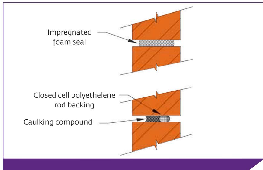
Figure 8. Methods of sealing control joints
