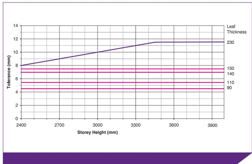
Figure 13. Structural tolerances for out of plumb (within each storey)
