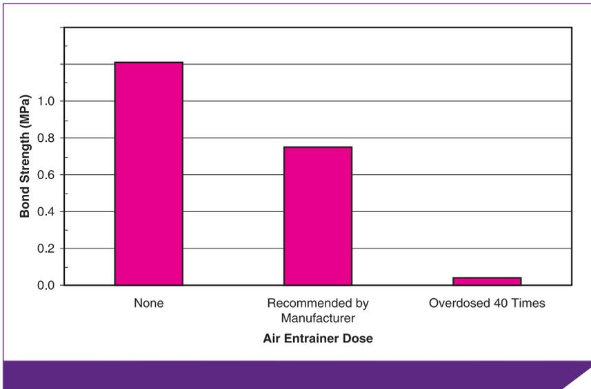
**Figure 4.** Typical effect of overdosing air entrainer
