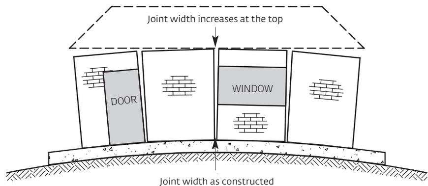
**Figure 8.** Effect of foundation movement on articulated walls (dishing foundation)
