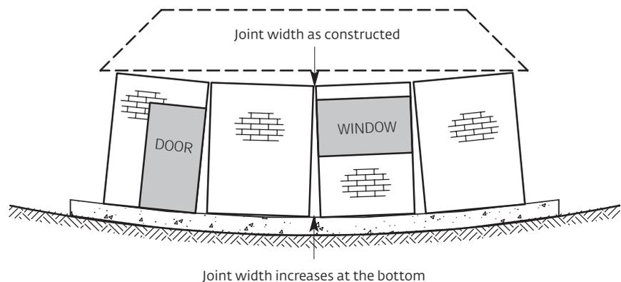
Articulation joints might also be required for internal walls. With good planning, the joints can be incorporated at full height openings such as doorways. Where joints are unavoidable, for example in long
