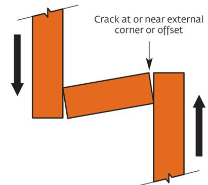
**Figure 5.** Oversailing of DPC caused by expansion
