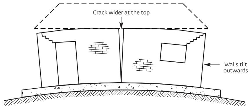
Figure 3. Typical cracking from a dishing foundation
