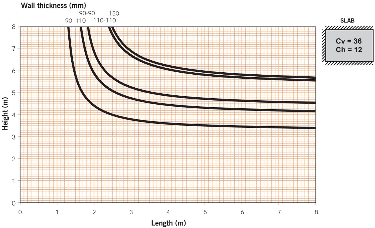
**Chart 5.** Robustness limits for clay masonry walls with one side free and loaded by other than a concrete slab
