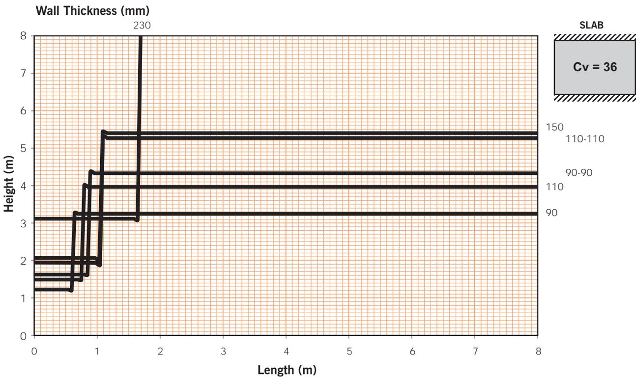
**Chart 8.** Robustness limits for clay masonry walls supported at top and bottom and loaded by other than a concrete slab
