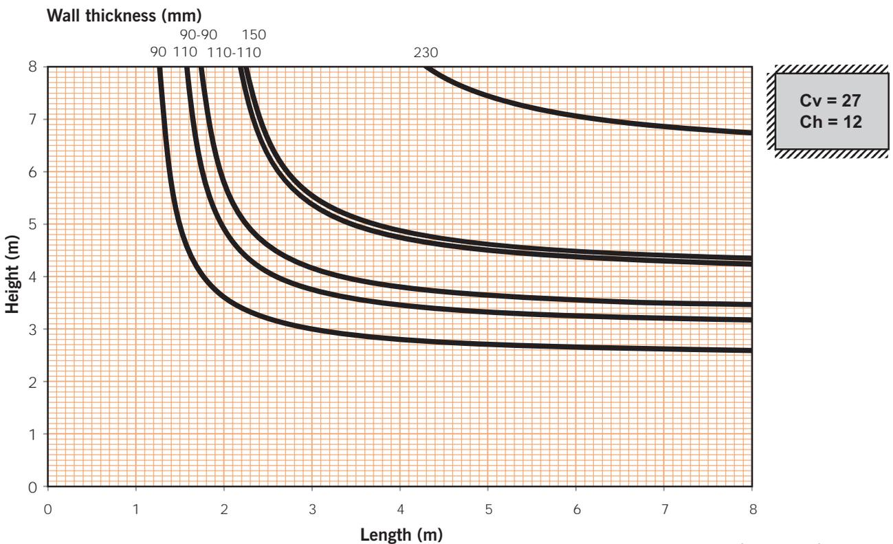
**Chart 6.** Robustness limits for clay masonry walls supported on two edges
