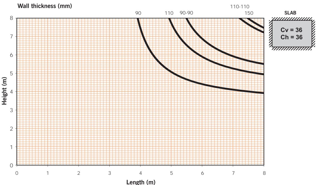
**Chart 4.** Robustness limits for clay masonry walls with one side free and loaded by a concrete slab
