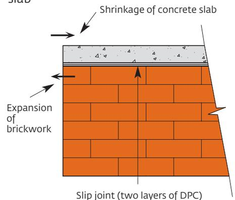
Where an isolation joint is necessary to isolate a wall from the surrounding structure, control joints can be used for this purpose. Flexible anchors such as those used for articulation joints should be incorporated across the joints if transverse wall loads have to be transmitted to a supporting frame.
