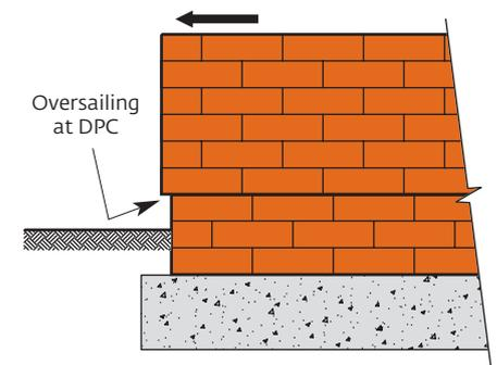
**Figure 6.** Failure of biscuit bricks caused by bowing and restrained expansion
