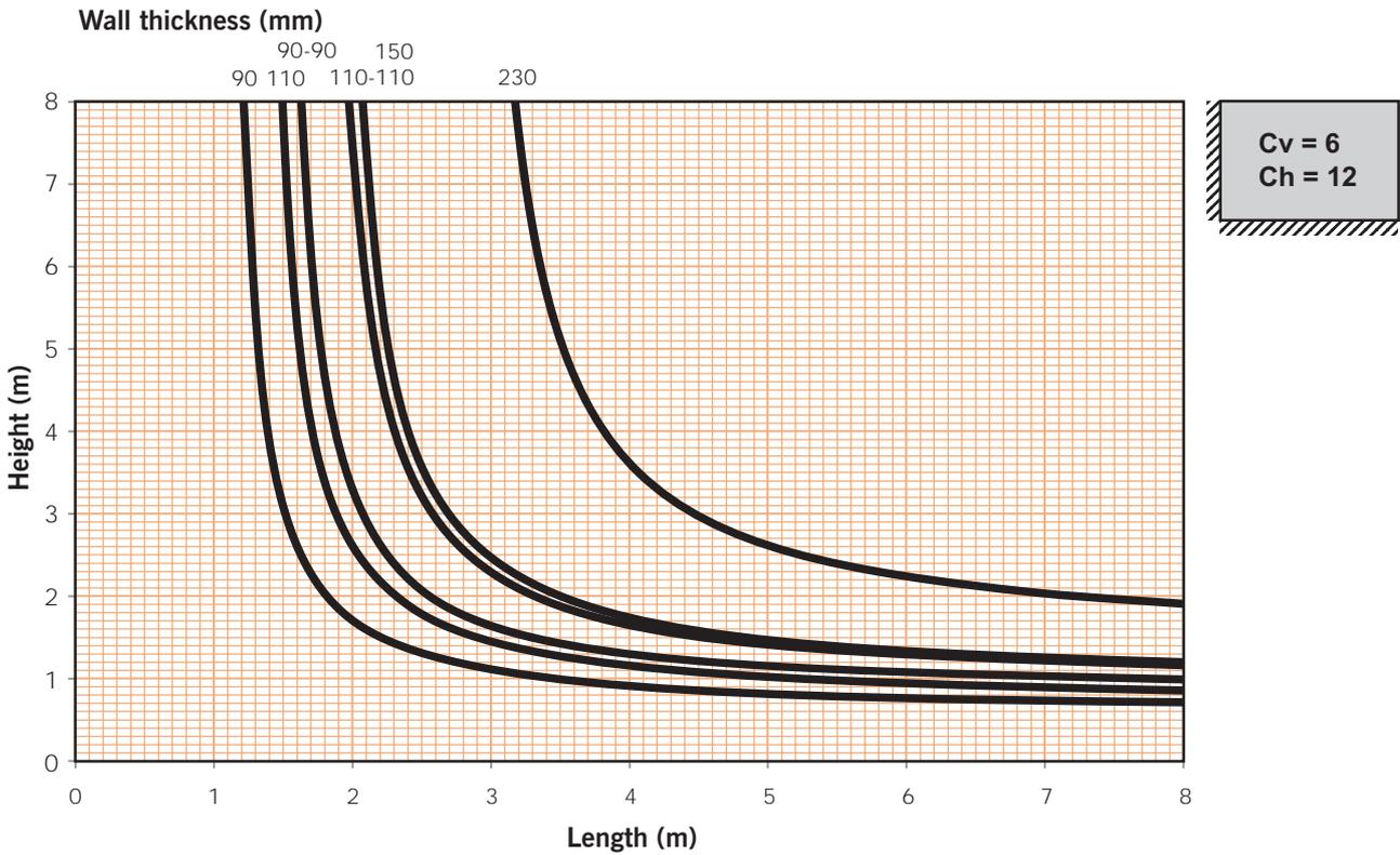
**Chart 7.** Robustness limits for clay masonry walls supported at top and bottom and loaded by a concrete slab
