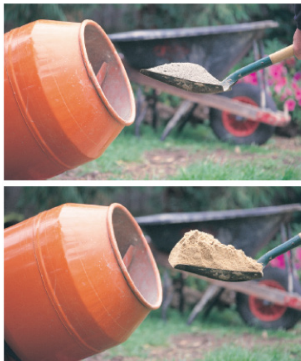
Figure 6. Effects of bulking on shovels of cement (top) and sand (bottom)
