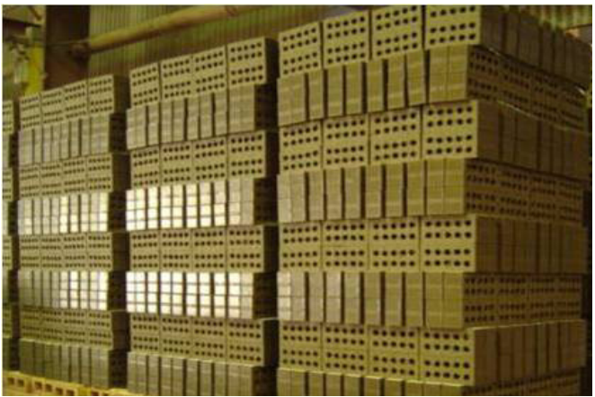
Figure 2.3 Drying of extruded bricks prior to firing
